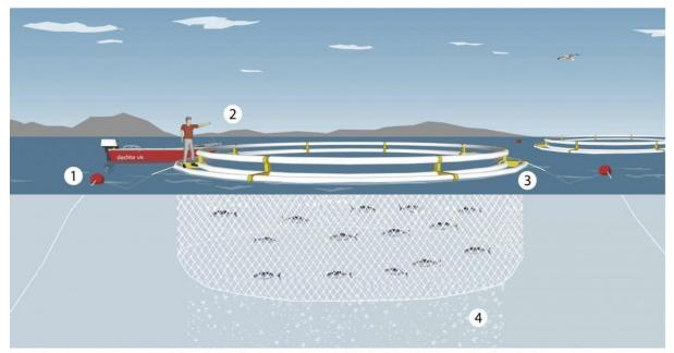
1. The cage is moored to the ocean floor 2. Fishemeal based feeds are added to the cages 3. Buoyant tubes keep the cages afloat 4. Fish faeces and waste fall through the cages
